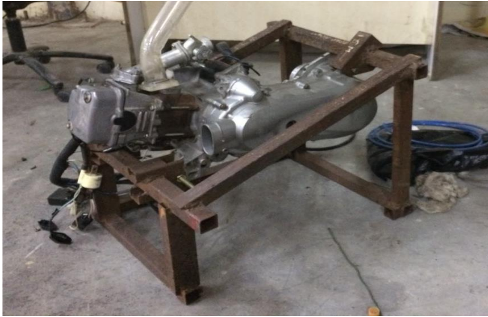
Figure 5.1: ENGIEN AND JIG AND INTAKE ASSEMBLY
